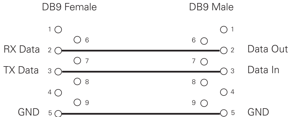
FIGURE 14-3. RS232 extension cable/connector wiring diagram
